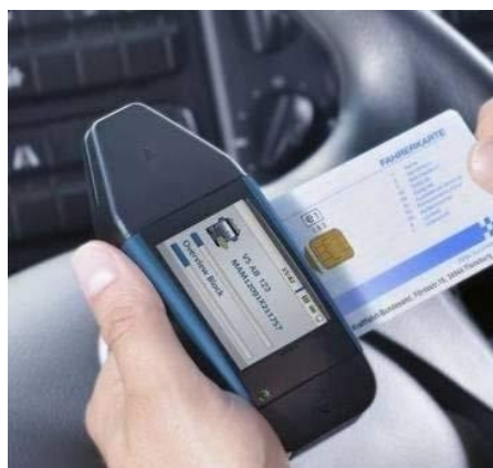
Figure 5. A smart device for tachograph analysis
