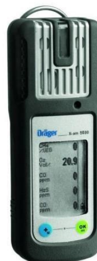
Figure 4. Device for measuring vapors from the tank
